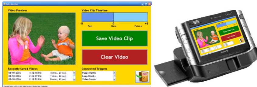
Figure 4: Left shows screen shot of smart baby monitor interface, which allows parents to save clips of recently experienced events. Right shows prototype developed on a Sony Vaio-U™
